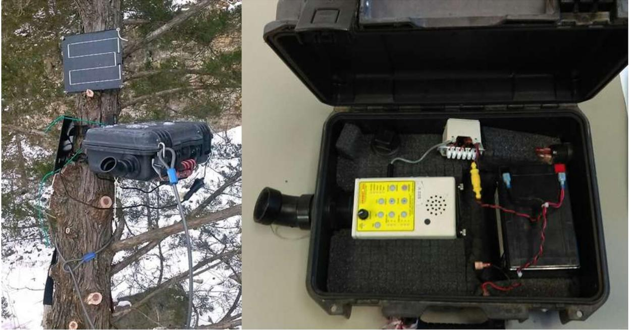
**Figure 1.** Example acoustic detector set up. Detectors were placed on trees or rocks with a 45° cone pointed upward toward possible bat flyways. Anabat detectors were powered with 12 volt batteries connected to either 1 or 2 solar panels.
