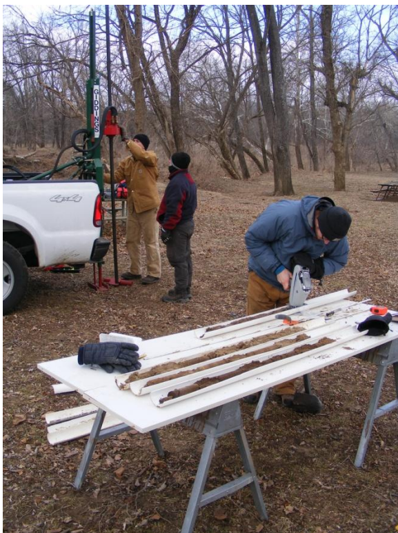
Figure 7B: Floodplain Sediment Sampling Coring floodplain deposits with Giddings probe and geochemical analysis with XRF
