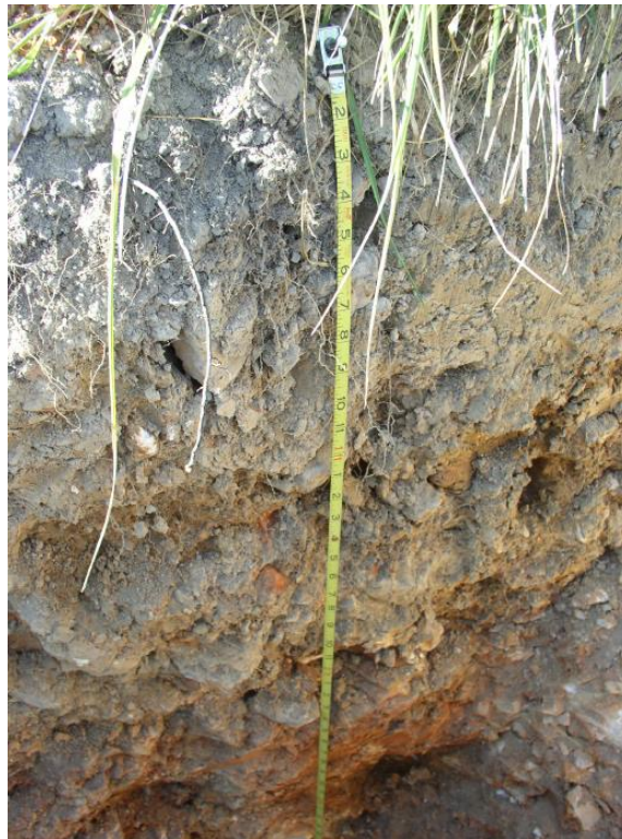
Photo 4. Soil pit #3 from the slightly steeper shoulder side slope with rocky colluvium over cherty red clay residuum.
