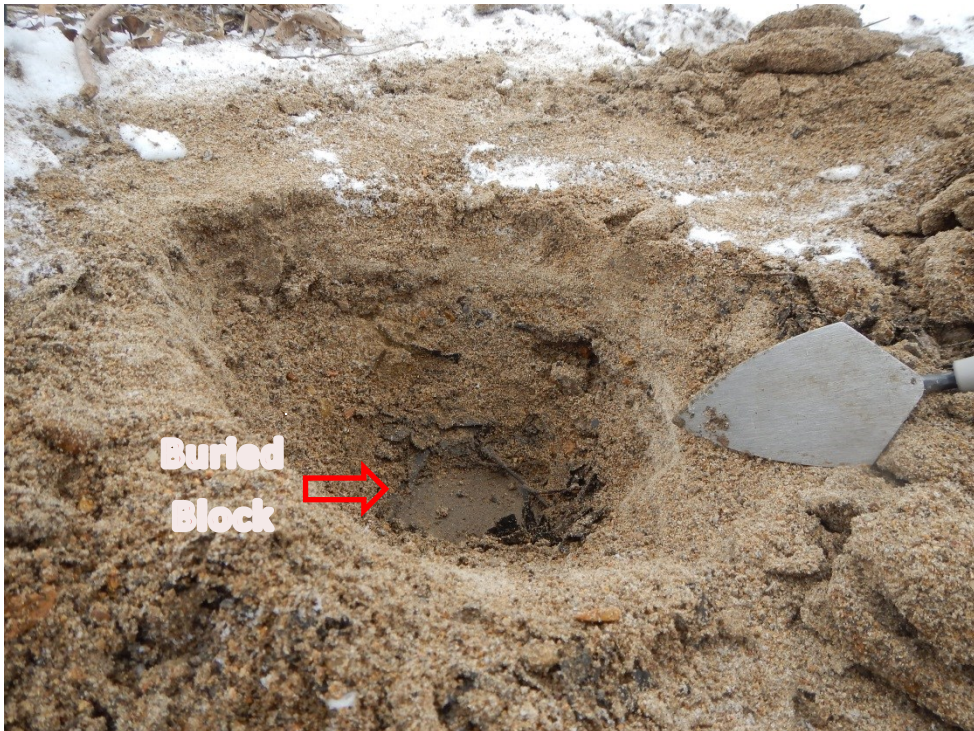
Photo 8. Sediment depth measurements and sample collection from block samplers (1/21/16).
