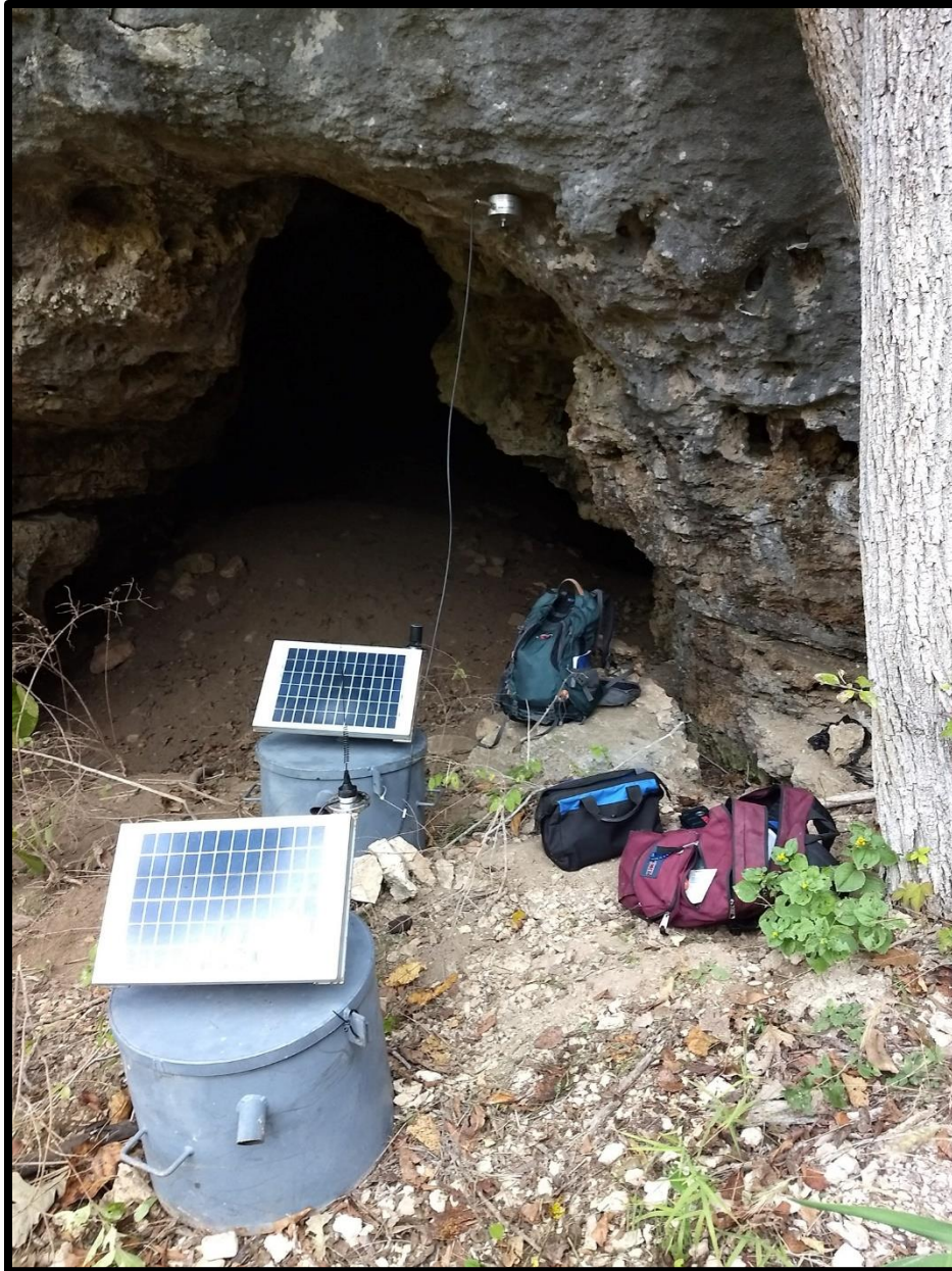
Figure 3. Seismic recorders at King Cave. The seismic sensor is attached to the top of the cave while the round containers contain the data recorders/batteries and solar panels. The sound meters were attached to the round containers.
