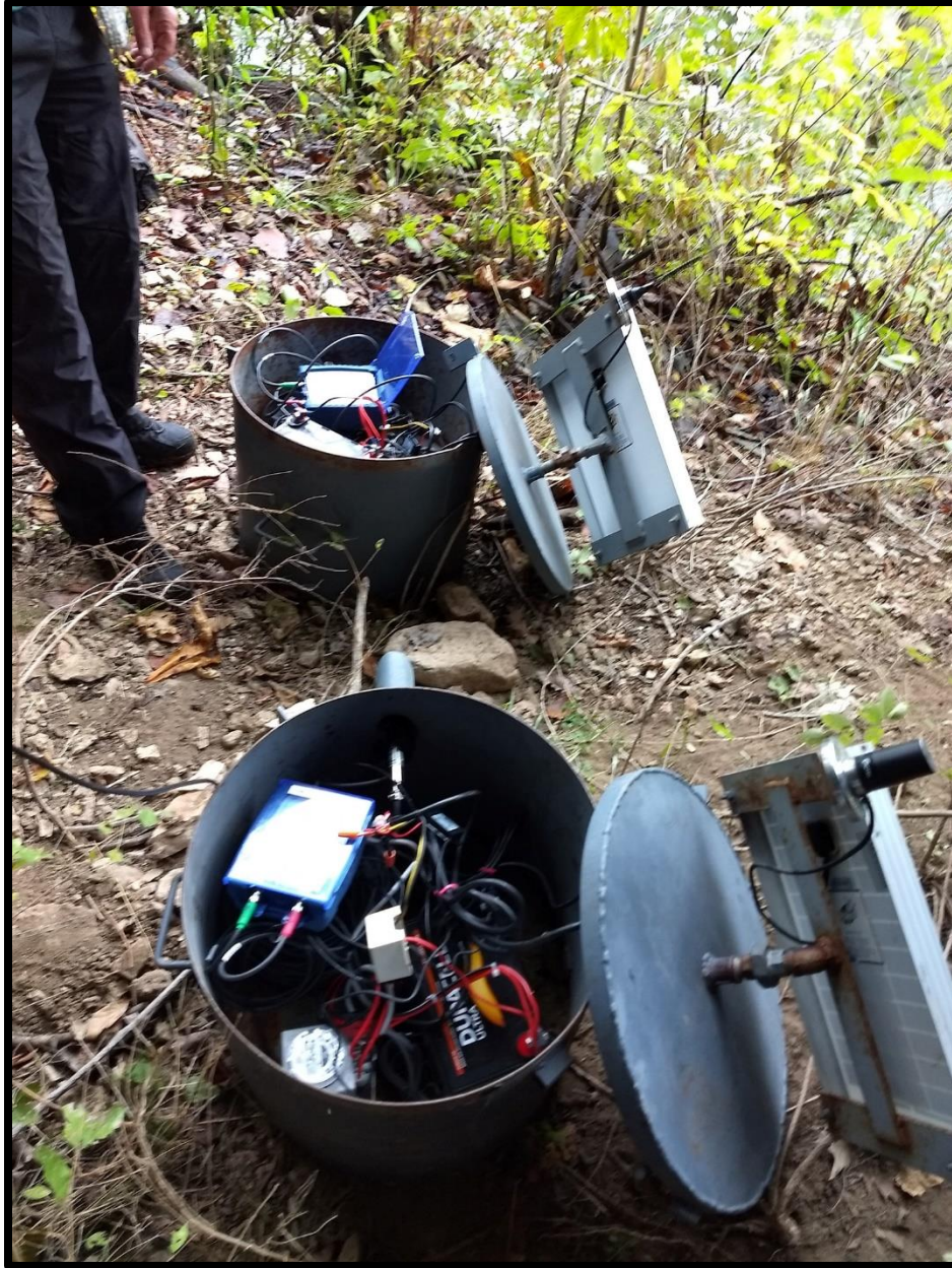
Figure 4. The data recorders (blue boxes) inside while the round containers. The sound meters were placed inside the round tube coming out of the containers (upper portion of the bottom container).
