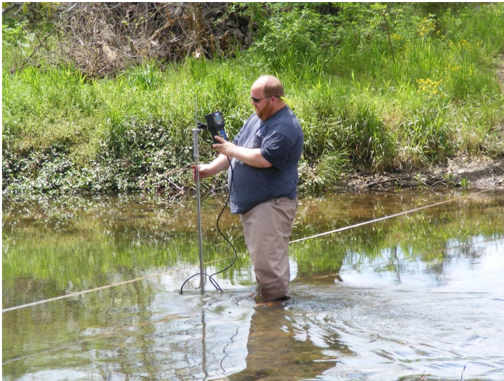
Photo 6. Discharge measurement using the FlowTracker ADP
