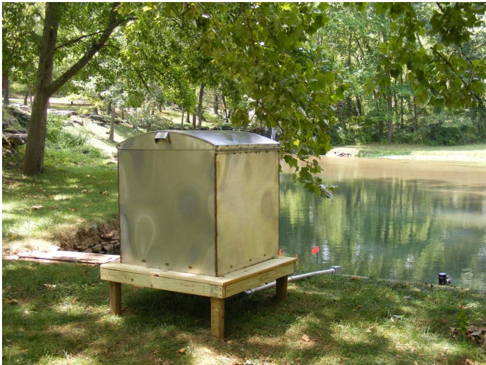
Photo 4. Sampler box installed in platform above the spillway at Site 2.
