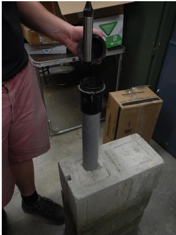
Photo 8. Levellogger removed from housing.
