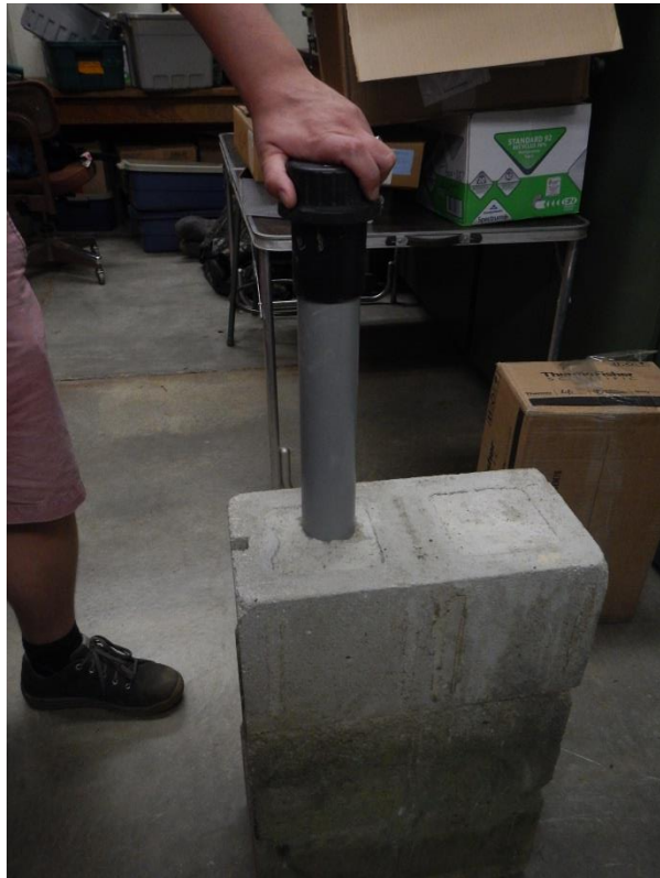
Photo 6. Levellogger housing with cap.
