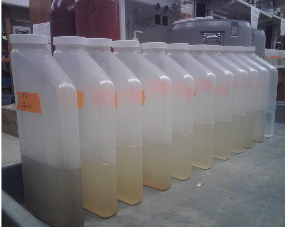
Photo 11. Line of 1-Liter Bottles after Split ready for Nutrient Analysis
