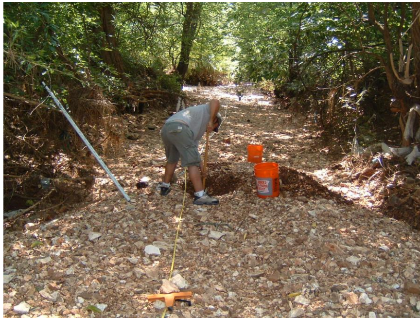
Photo 2: Sediment being collected for tracer experiment
