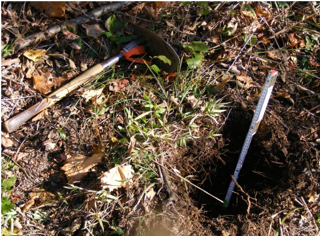
Figure 7. Floodplain soil sampling. Top shows the typical location of floodplain deposits sampled in 5-10 cm intervals from the surface to the depth of buried gravel deposits. Bottom shows a sample pit on a floodplain.
