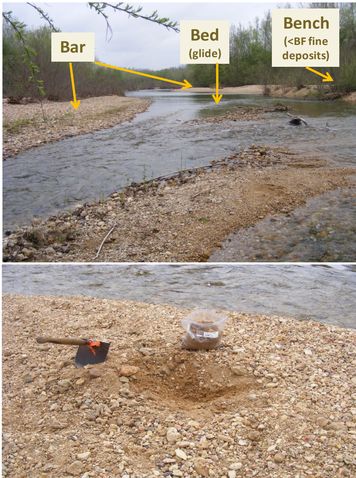
Figure 4. In-channel sediment sampling. Top shows the typical locations of three different types of sediment deposits. Bottom shows the texture of a typical channel bar surface and shallow sample pit with bagged sample ready to be transported to the laboratory. Note the coarser armored layer at on the bar surface and the finer sediment below that is more representative of the bar material as a whole.
