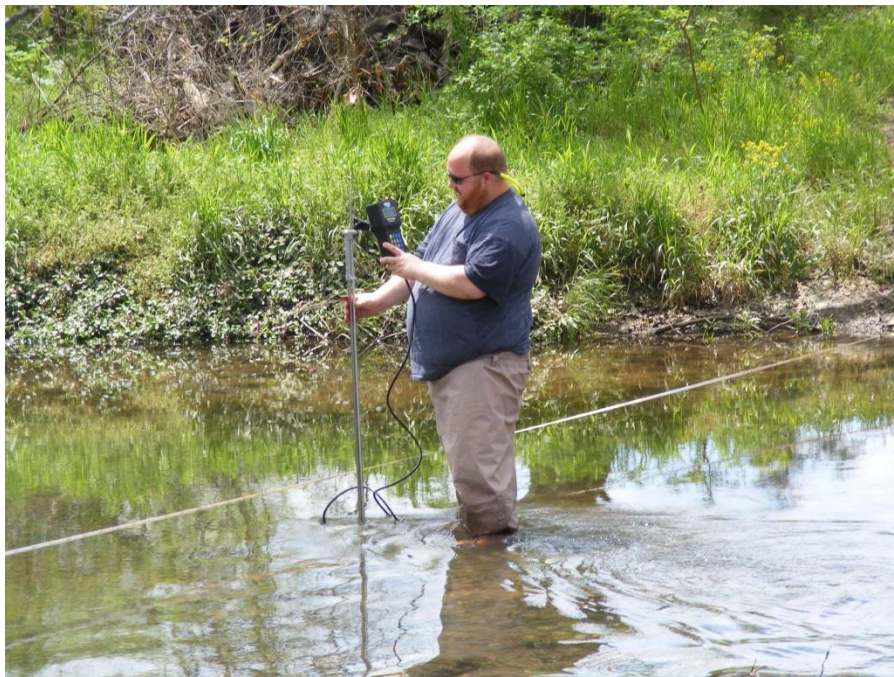
Photo 8. Discharge measurement at site AC06 using the FlowTracker
