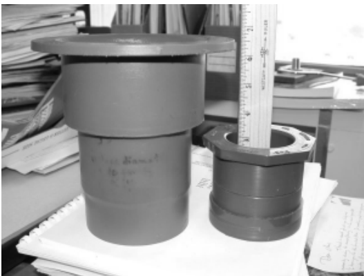
Figure 3. A) Venturi and venturi bushing inserts. B) Venturi assembly welded to the base of the tank.
