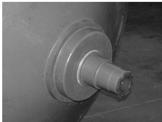
Figure 3. A) Venturi and venturi bushing inserts. B) Venturi assembly welded to the base of the tank.
