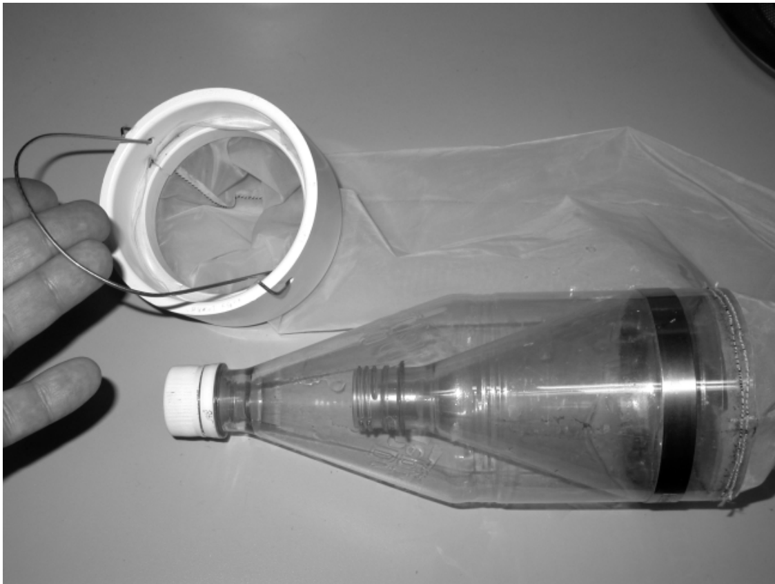
Figure 7. Recovery filter diagram and photograph. The net bag is 125 micron mesh Nitex cloth*. The hoop is a 3-inch PVC coupling cut in half, with a split ring of 3-inch PVC nested into the coupling to hold the end of the bag. The cod end is made of the cut-off ends of two 1-L plastic soda bottles. One cut-off end (the cod end insert) is nested inside the other (the cod end bottle) and secured with a hose clamp. The net bag is sewn to the cod end bottle.
