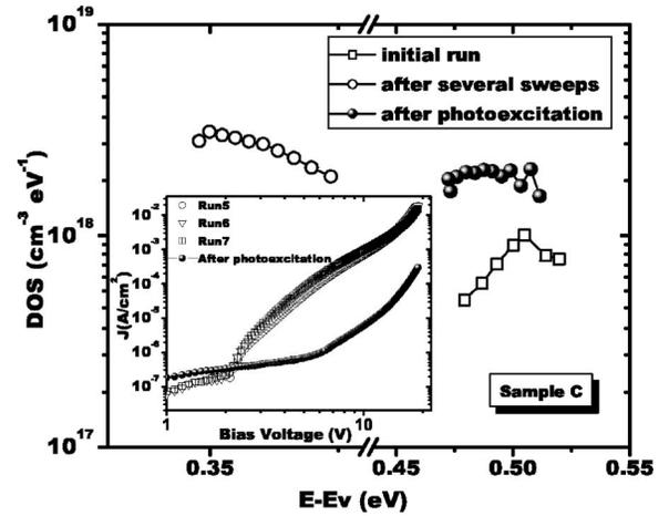
FIG. 2. DOS distribution as a function of the quasi-Fermi level for the initial, trap-filled, and after photoexcitation bias sweeps in sample C. The inset shows successive  $J$ - $V$  curves after running the device many times. The bottom curve in the inset was measured after photoexcitation.
