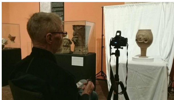
Figure 17. Photogrammetric capture process of the exhibited pieces by using the ComXim Professional 360 Degree photography turntable, Cannon Rebel EOS T3 with shutter remote control and portable sets of lights and backdrops.
