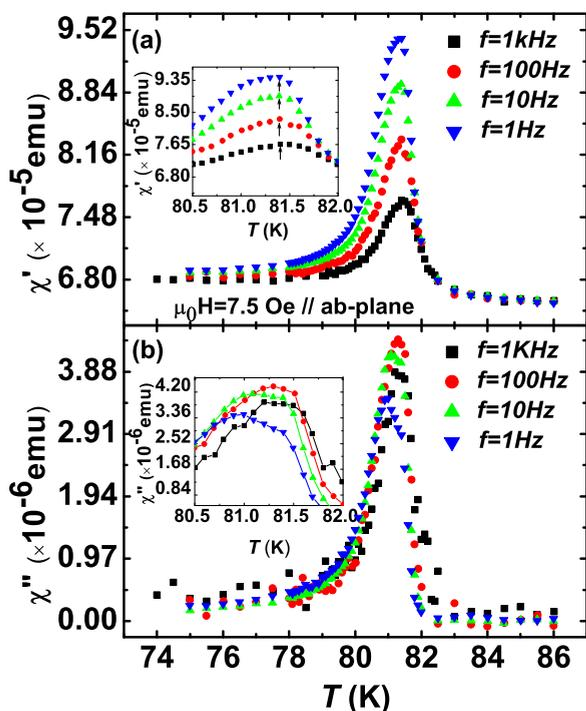
FIG. 3. (Color online) Real ( $\chi'$ ) (a) and imaginary ( $\chi''$ ) (b) components of the ac susceptibility of the  $\text{YBaCo}_4\text{O}_{7.1}$  single crystal as a function of temperature and frequency in the range 1–1000 Hz with an ac field of 7.5 Oe and zero dc field. The peak at  $\sim 81$  K corresponds to the cusp in the magnetization results shown in Fig. 2. The insets show an expanded  $T$  scale.
