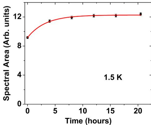
FIG. 6. (Color online) Evolution of the  $^{59}\text{Co}$  ZF NMR spectral area with time for the NS  $\text{YBaCo}_4\text{O}_{7.1}$  crystal following fast cooling from 290 to 1.5 K. The fitted curve shows exponential growth with a characteristic growth time of 3.3 hours for the particular conditions used.
