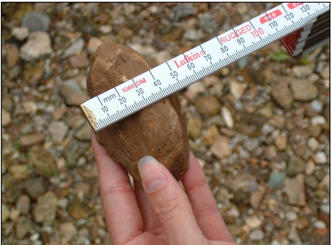
Figure 4.7 Measurement of the b-axis of a sediment sample
