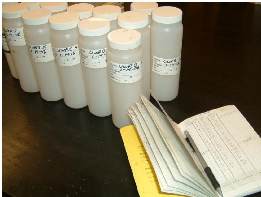
Figure 3.1: Labeled sample bottles. Containers used for water quality grab sampling
