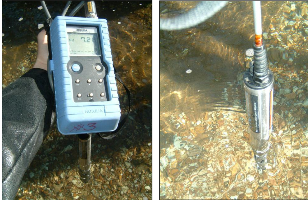
Figure 3.2: Horiba U-22. Unit displays digital readout screen (left) and probe (right)
