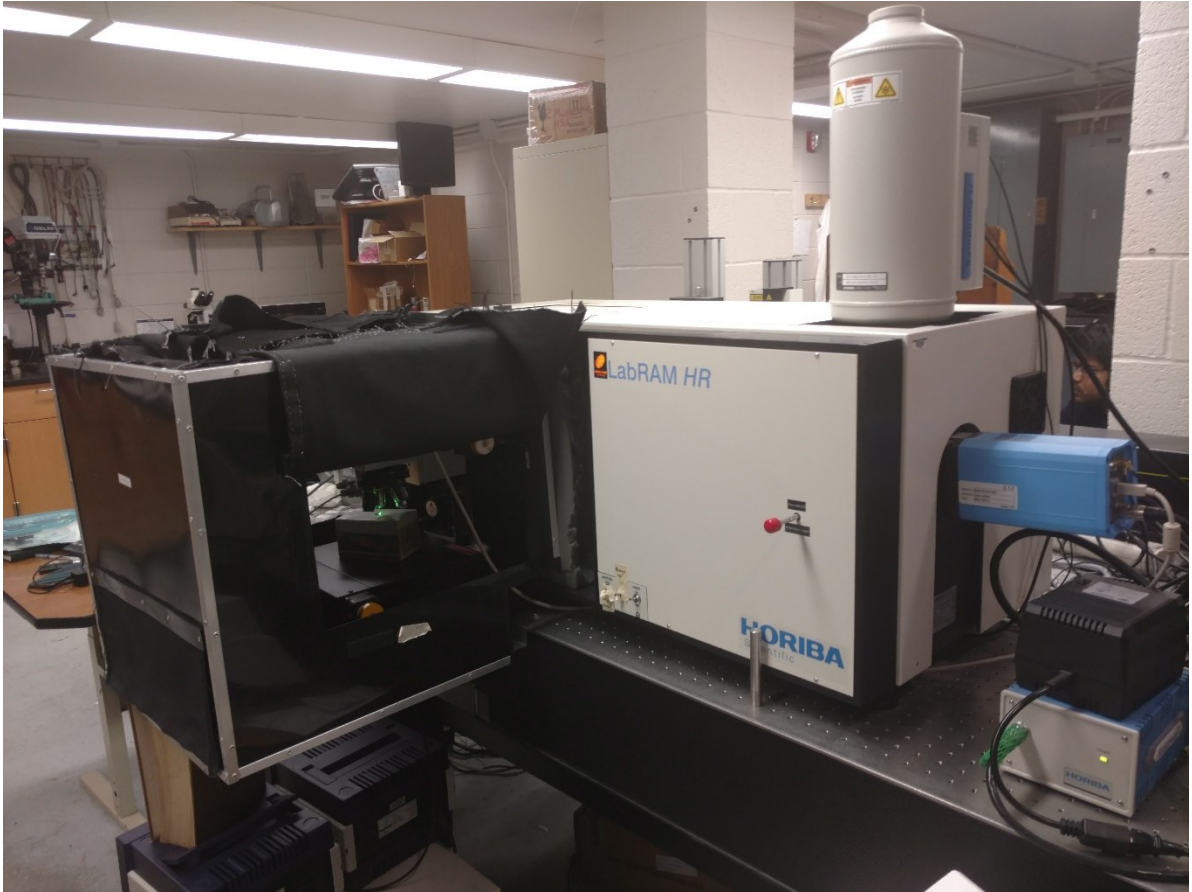
Figure 3.1: Horiba LabRAM HR 800 Evolution Raman spectrometer.
