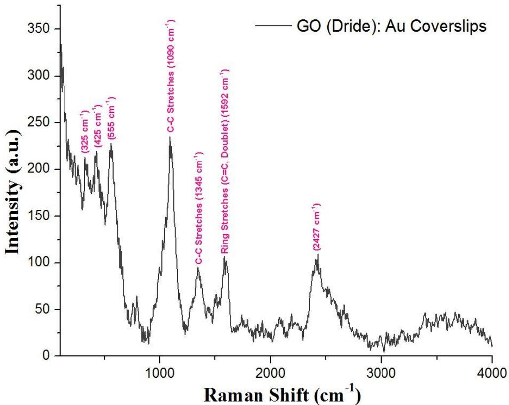
**Fig. 4.18** Raman spectrum of dried graphene oxide solution on an Au coated glass slide (100-4000  $cm^{-1}$ )
