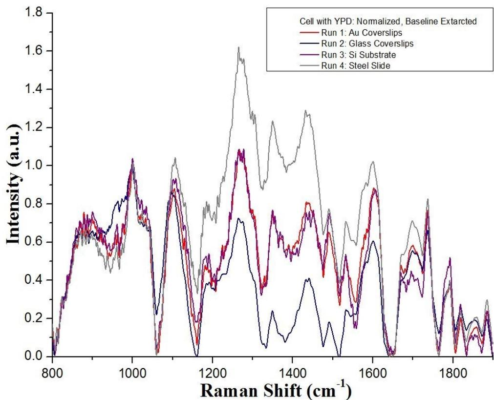
**Fig. 4.23** Baseline extracted and normalized Raman spectra of yeast cells with YPD medium ( $800\text{-}1900\text{ cm}^{-1}$ ) from Fig. 4.21
