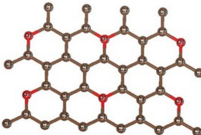
**Fig. 4.8** An oxidized graphene structure with defects obtained by replacing C atoms with O atoms. Note that the brown and red lines indicate symmetry of the initial structure, and not actual covalent bonds between the atoms
