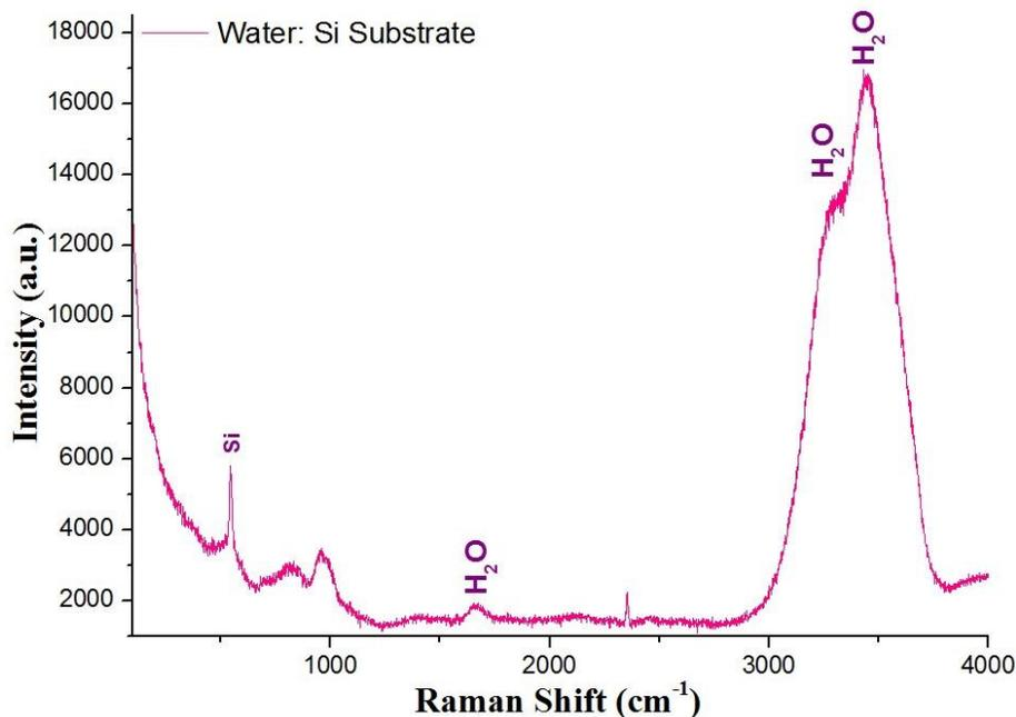
**Fig. 4.3** Raman spectrum of pure water on Si substrate (50-4500 cm<sup>-1</sup>)
