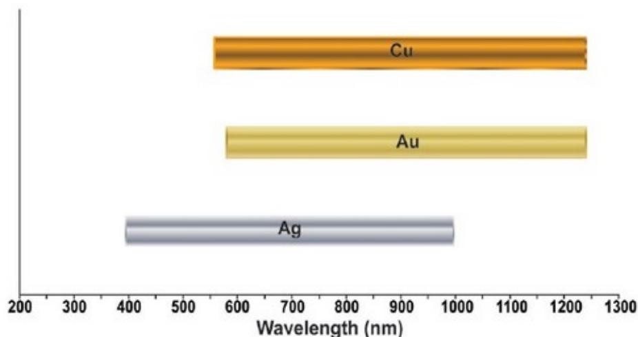
**Fig. 2.4** Approximate wavelength ranges where Ag, Au, and Cu nanostructures show LSPR absorption of light; reproduced with permission of Elsevier <sup>42</sup>
