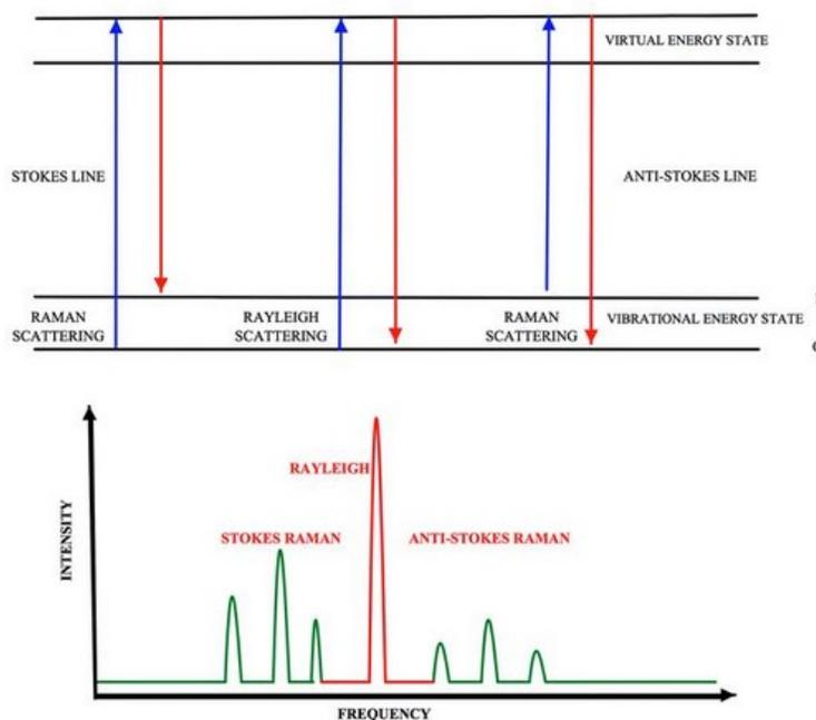
**Fig. 2.1** Energy level diagram of Raman and Rayleigh scattering; reproduced with permission of Royal Society of Chemistry<sup>27</sup>
