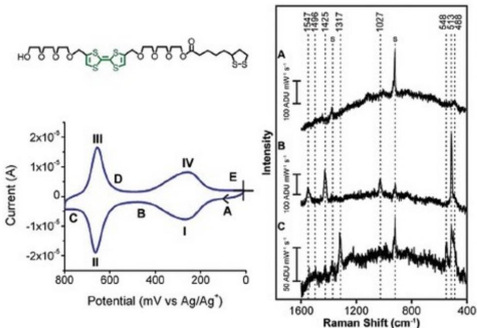
**Fig. 2.6** Spectroelectrochemistry of a tetrathiafulvalene -derivative. Top left: molecular structure; bottom left: cyclic voltammogram in acetonitrile on a gold film over nanopsheres; right: surface-enhanced Raman spectra at different potential; reproduced with permission of Elsevier <sup>44</sup>
