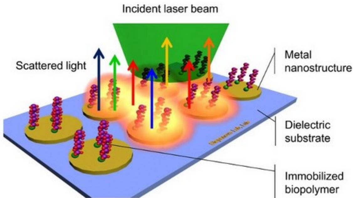
**Fig. 2.3** Scheme of surface-enhanced Raman spectroscopy; reproduced with permission of JoVE <sup>41</sup>
