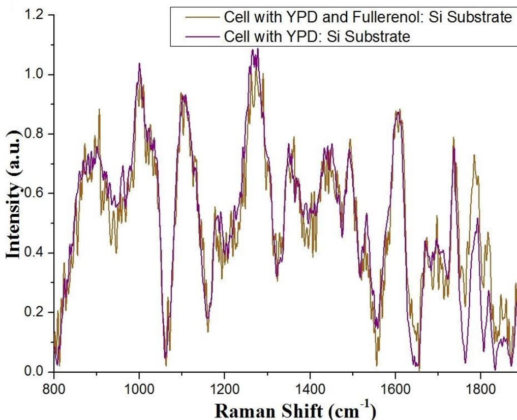
**Fig. 4.25** Comparison of Raman spectra for yeast cells in YPD medium with fullereneol added, and cells in YPD medium on Si wafers (800-1900  $\text{cm}^{-1}$ )
