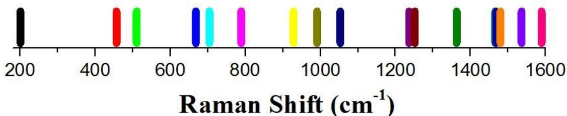
Fig. 4.13 Predicted Raman bands of oxidized graphene with defects (C<sub>7</sub>O) (200-1600 cm<sup>-1</sup>)
