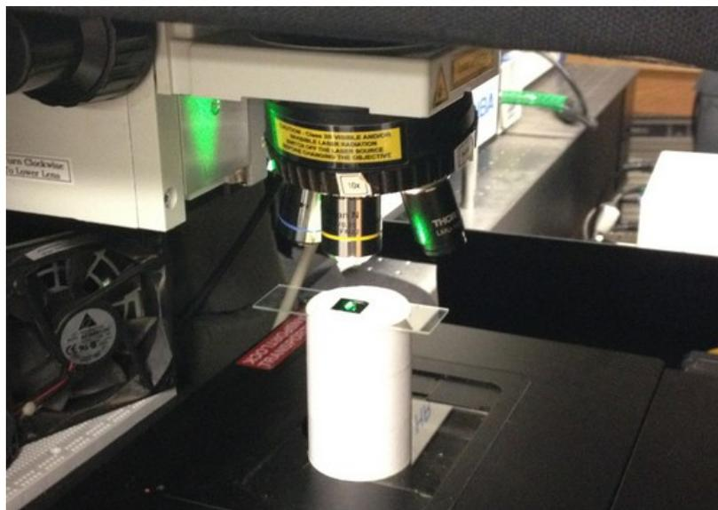
**Fig. 4.2** Sample area of the LabRAM HR800 instrument.
