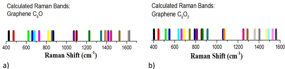
**Fig. 4.15** Predicted Raman bands of C/O models: (a) - 8:1 (400-1700 cm<sup>-1</sup>) and (b) - 8:2 (400-1600 cm<sup>-1</sup>)
