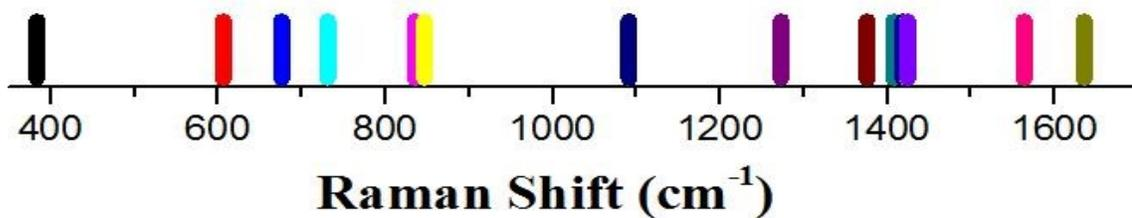
Fig. 4.12 Predicted Raman bands of Graphene (C<sub>8</sub>) (300-1650 cm<sup>-1</sup>)
