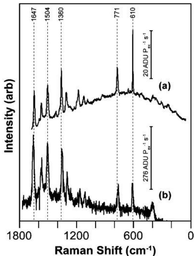
**Fig. 2.7** Representative single-molecule SERS spectra of rhodamine 6G on silver obtained using a 532-nm excitation. (a) - Ensemble-averaged SERS obtained on an Ag island film and (b) single molecule SERS spectrum obtained on a colloidal Ag aggregate; reproduced with permission of Elsevier<sup>47</sup>
