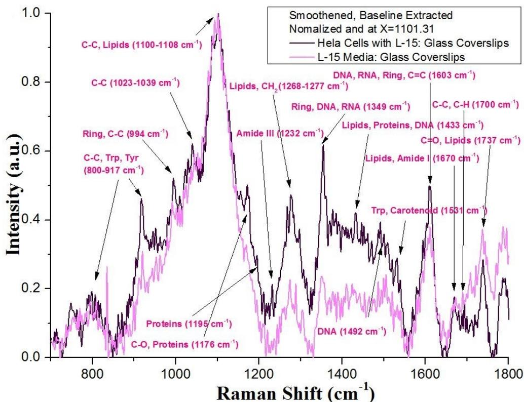
**Fig. 4.29** Baseline-extracted and normalized Raman spectra of HeLa cells with L-15 medium and L-15 medium alone on glass coverslips with band assignments (700-1800  $\text{cm}^{-1}$ )
