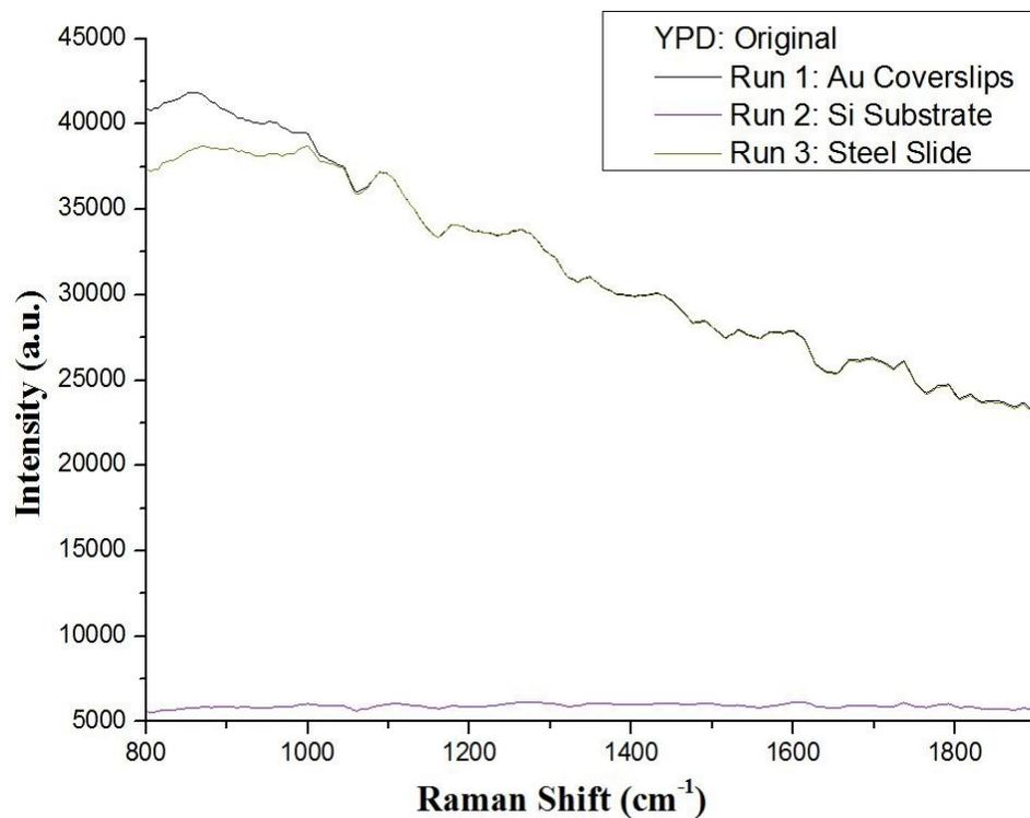
**Fig. 4.4** Raman spectra of YPD media (a biological sample) on different substrates (800-1900 cm<sup>-1</sup>)
