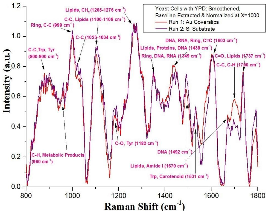
**Fig. 4.26** Raman spectra of yeast cells in YPD medium on Au-coated glass coverslip and Si wafer with band assignments (800-1800  $\text{cm}^{-1}$ )
