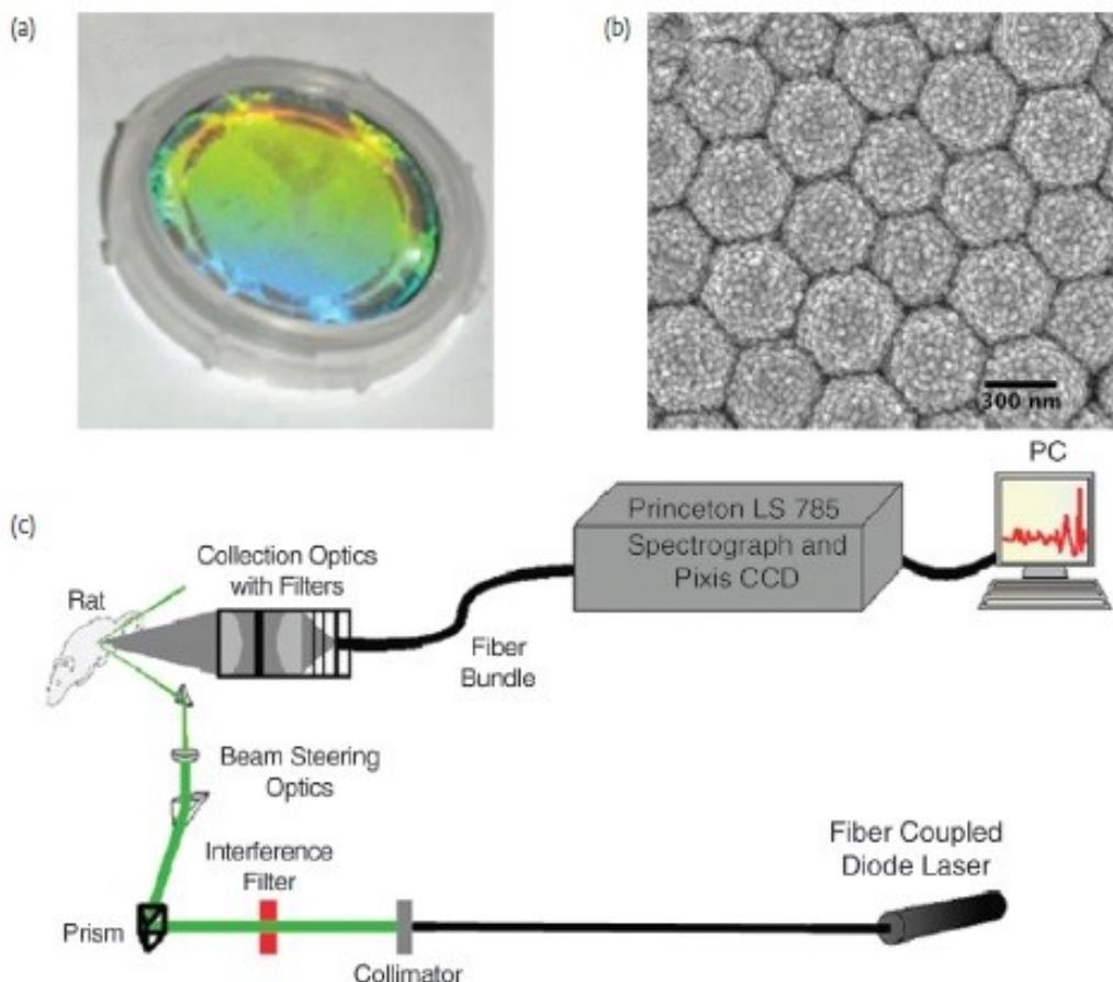
**Fig. 2.5** (a) - Silver film (200nm) over 880 nm Si nanospheres (AgFONs) on an 1-inch glass coverslip; (b) - SEM image of the system; (c) - Schematic of the acquisition apparatus; reproduced with permission of Elsevier<sup>43</sup>
