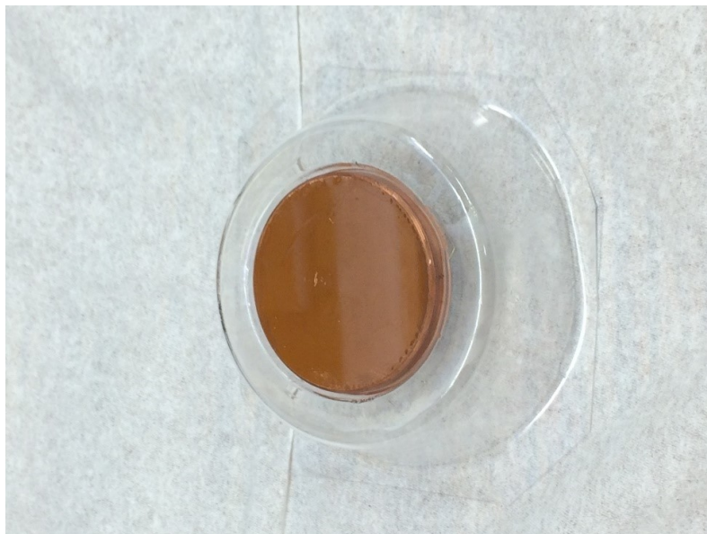
Figure 15. Copper mirror used as flag within the system. (Michal Bulak)
