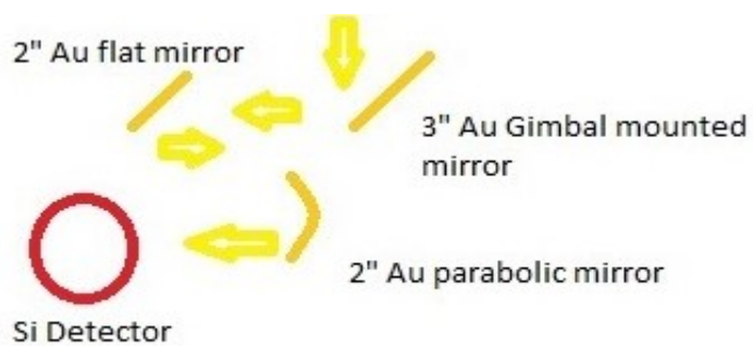
Figure 16. Optical pathway exiting the chamber. (Heath Gemar)
