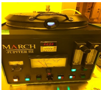
Sputtering carried out by fixing up parameters that ensures a 10 nm/min deposition
