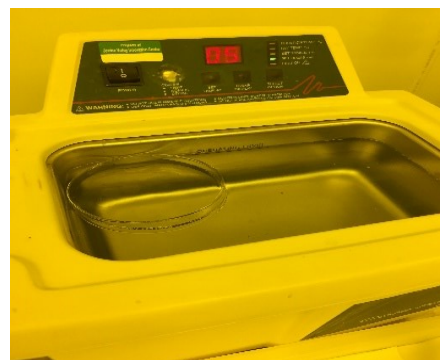
Acetone sonication for 5 mins.
