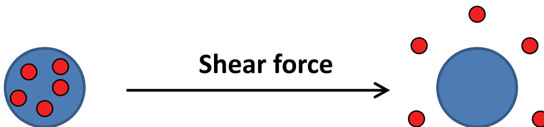
Figure 2. Micelle (blue) with encapsulated hydrophobic FRET pair (red). The hydrophobic material is released in response to a shear force.
