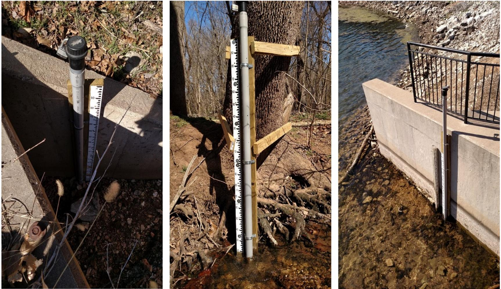
Figure 19. Continuous stage gages installed at sites FR-102, SS2, and RD
