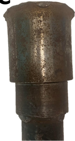
Appendix A-5. The cap (A), the collar of the tube (B), and the cap placed on top of the tube (C).
