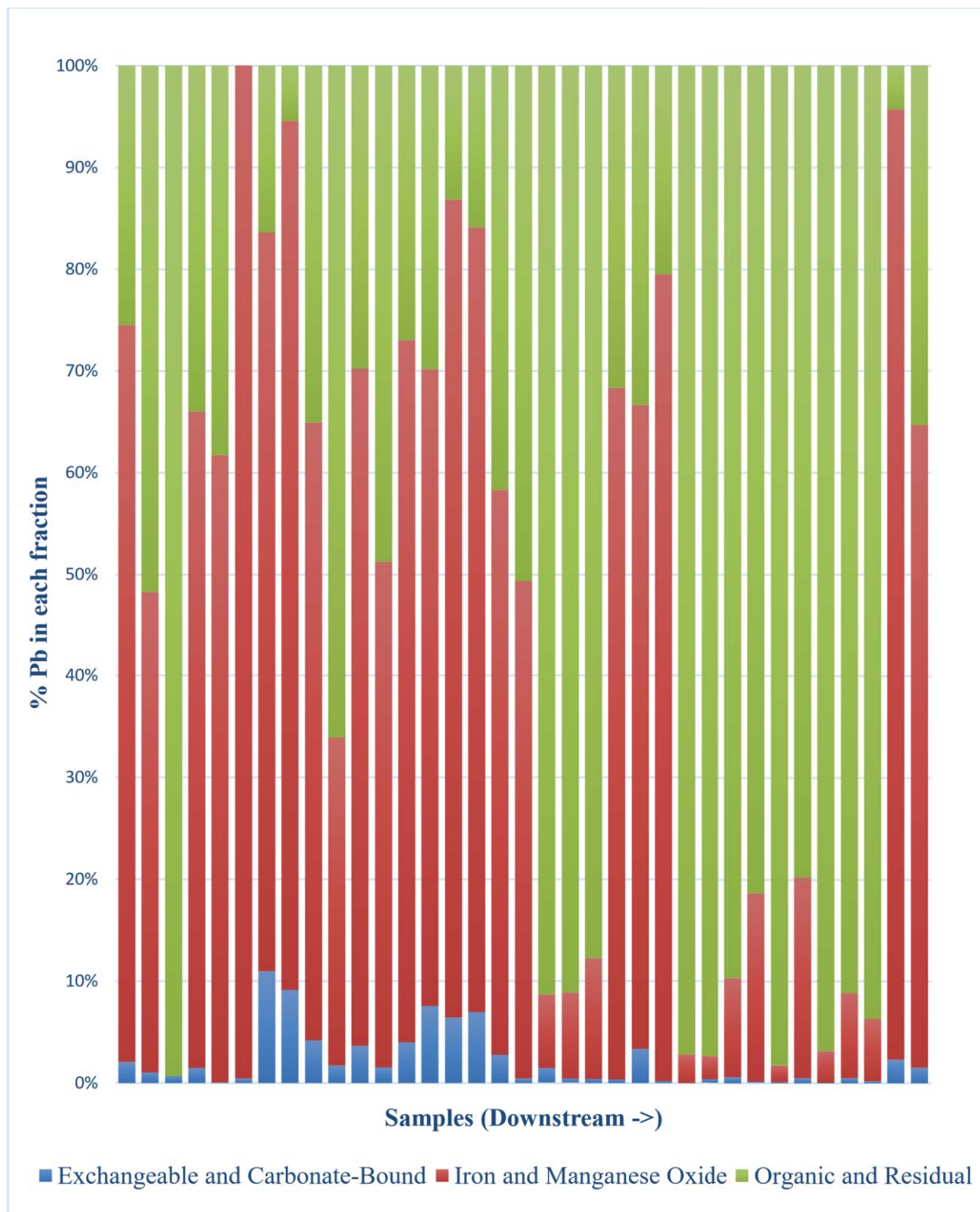
Figure 16 - Lead concentrations in exchangeable and carbonate-bound, iron and manganese oxide, and organic and residual fractions of sediment expressed as a percentage of the total lead concentration.
