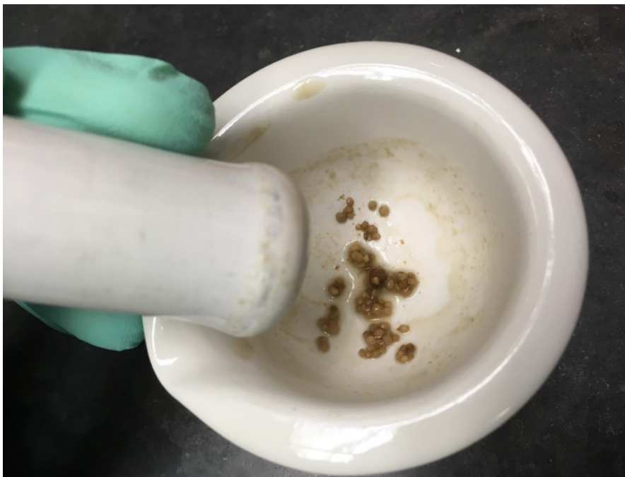
Figure 11. Nodules were ground with mortar and pestle
