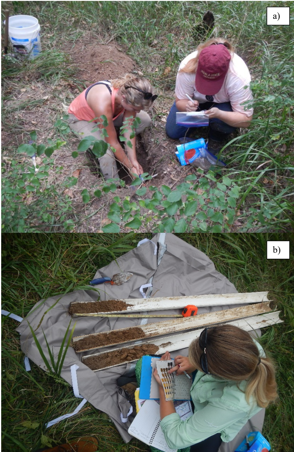
Figure 15. Examples of soil sample collection. Figure 17-a shows the collection of soil via pit sampling at the Lower Big Barren 101718 site. Figure 17-b is an example of soil core analysis in the field using soils cores from the Giddings soil corer at the Nature Conservancy site 1.
