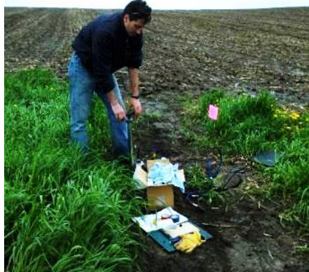
Figure 3. Soil water nitrate collection from a continuous corn grain site (OM70/90). The sampling port was located in a grassed waterway.
