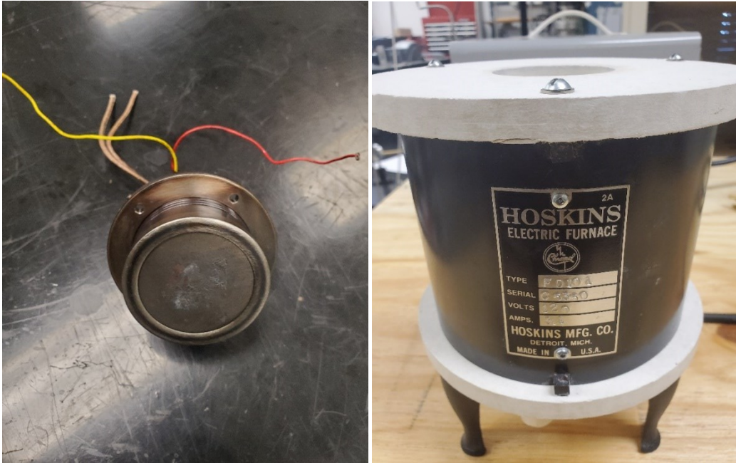
Figure 2.9 Resistive heater and vertical furnace
