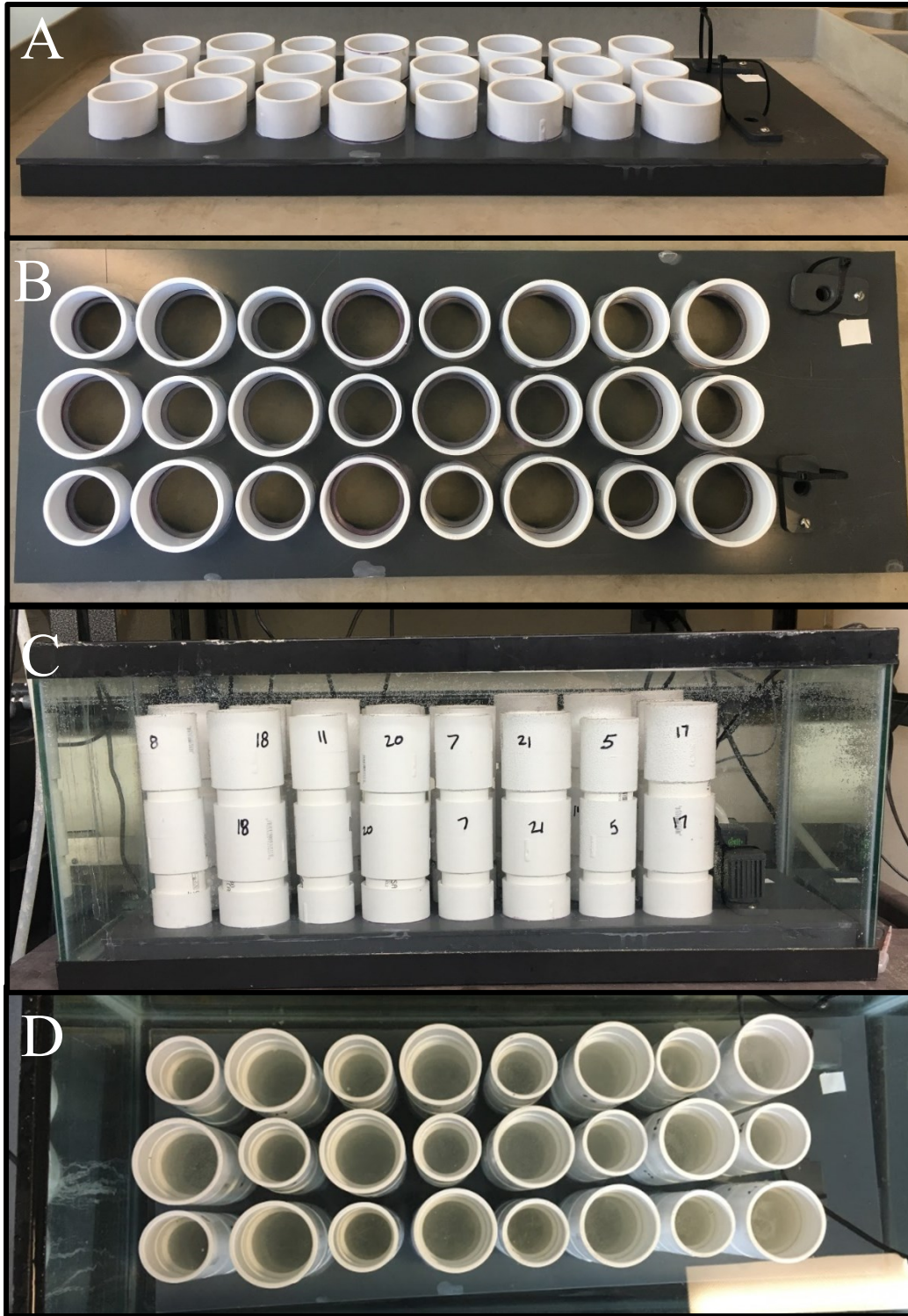
Figure 1. Aquarium assembly for survival and growth experiments. (A) Lateral view without chambers inserted. (B) Dorsal view without chambers inserted. (C) Side view of aquarium with chambers inserted into the false bottom floor. (D) Dorsal view of aquarium with chambered inserted into the false bottom floor.
