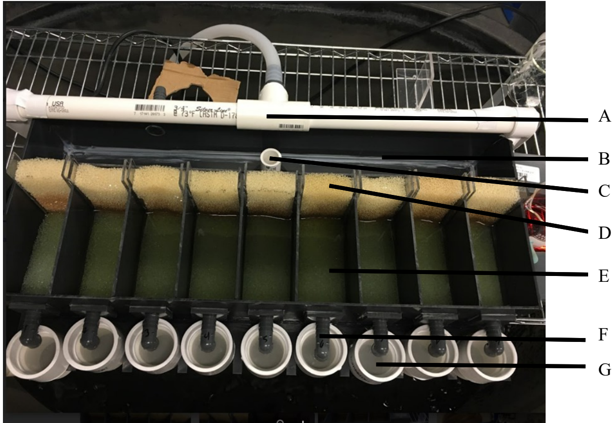
Figure 3. Flume for drift experiments. Manifold (A) delivers water to header box (B). Header box contains a standpipe (C) to allow exit of water and control water level. Header box has openings (not visible) to admit water into each lane. Foam baffles (D) over each opening rectify flow into the lanes, which contain 2.5 cm-deep substrate (glass beads (E)). An outflow fitting (F) from each lane conducts water into the filter cups (G) for recovery of drifting juveniles. The flume was constructed of 1/8 in polyvinyl chloride (PVC) sheet. The header box measured 57.2 cm long by 7.6 cm wide by 10 cm deep. Filter cups consisted of 150 \mu\text{m} Nylon screening press fit between a 3.8 cm (inside diameter) coupling and a piece of pipe. The entire assembly was supported over a water reservoir and pump to maintain recirculating flow (see Methods).
