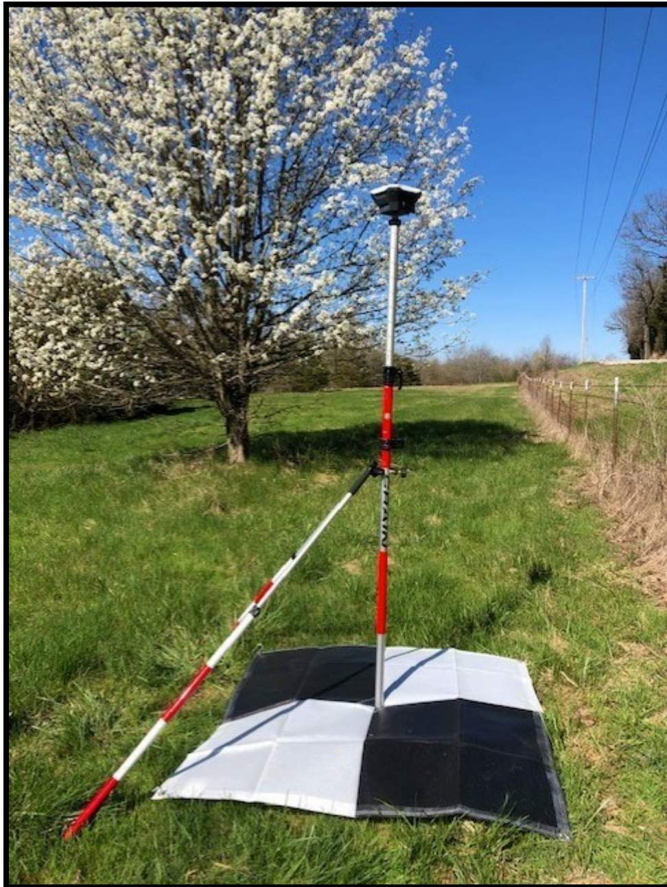
Figure 10. Rover stationed over a GCP collecting data at Fellows Lake
