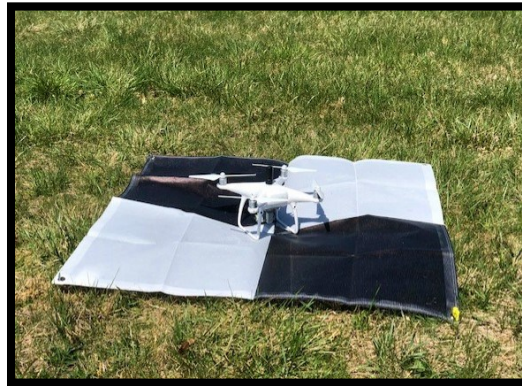
Figure 2. Canvas Ground Control Point in the Field Used for Georeferencing
