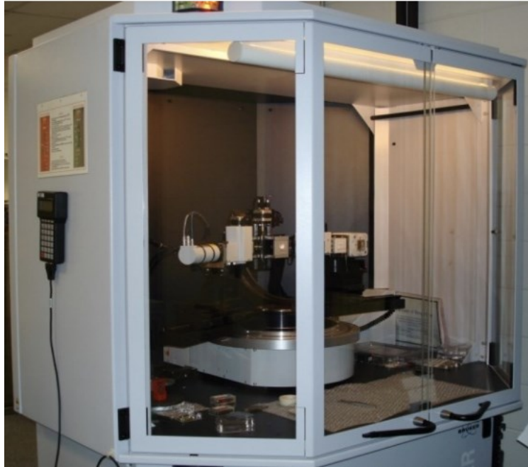
Figure 2.9. The set up for XRD machine used in the lab
