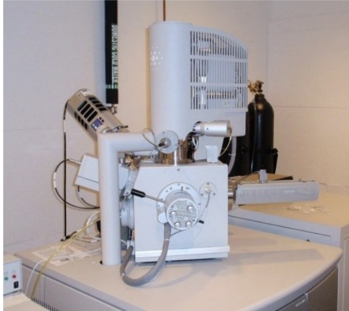
Figure 2.11. The FESEM set up for the experiment
