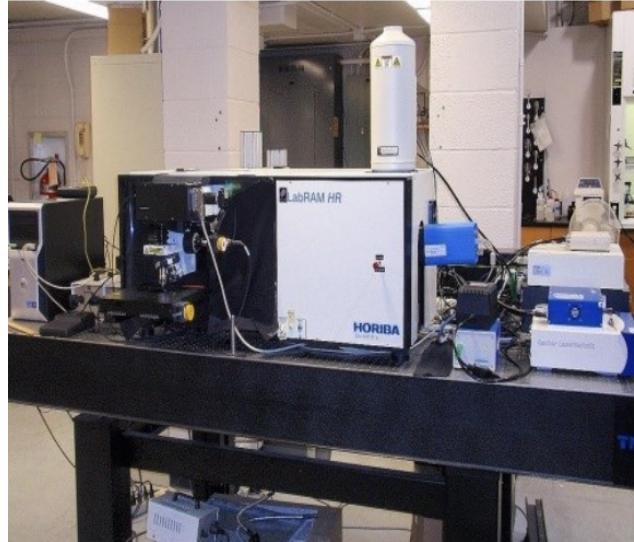
Figure 2.10. The set up for the Raman-PL spectroscopy
