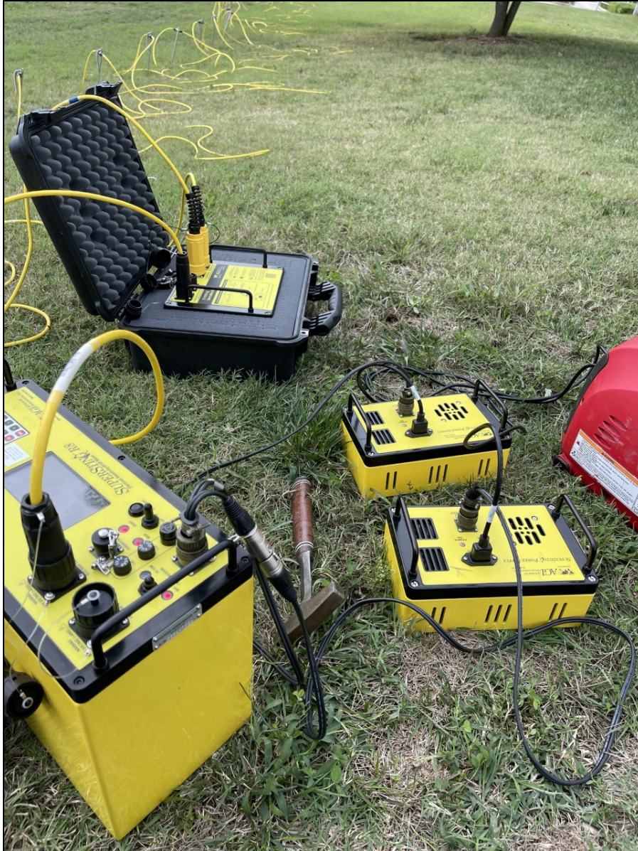
Figure 28. Supersting R8 set up in the field.
