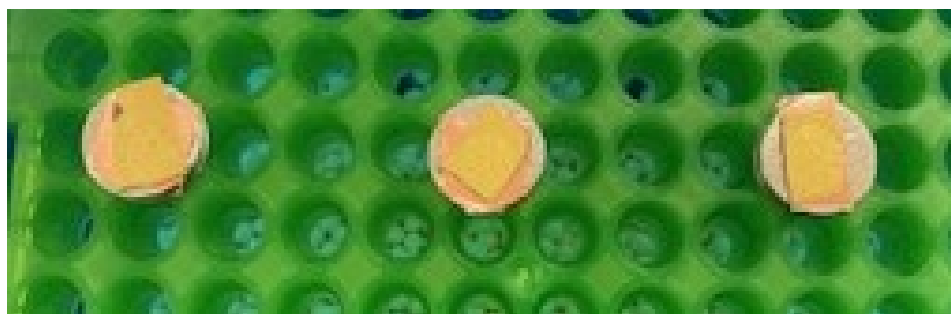
Figure 11. CD samples for SEM-EDS analysis. CD samples are dropcast onto gold-coated silicon wafers attached to aluminum stubs with copper tape.
