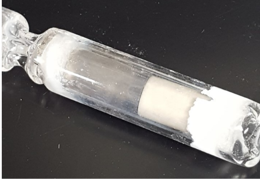
Figure 2.5 A fully sealed reaction ready for the furnace. The bottom alumina crucible contains the chemicals and the top crucible contains quartz wool that will act as a filter.
